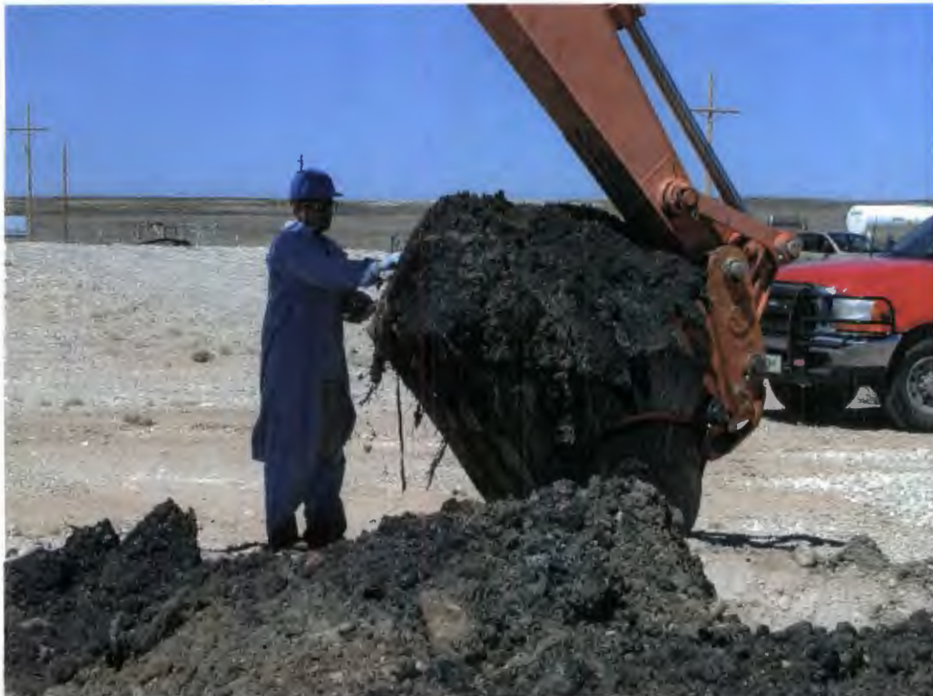
Collecting a sample for lab analysis from a trench in the Pit #1 area.
