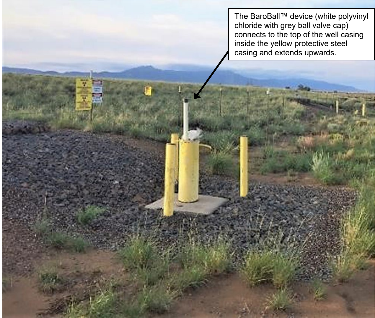
Figure 2-8 Photograph of a BaroBall™ Passive Venting Device on Groundwater Monitoring Well MWL-MW9 on the Western Perimeter of the Mixed Waste Landfill
